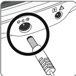
**b** Plug the small end of the power cord into the adaptor socket on the side of the device.
